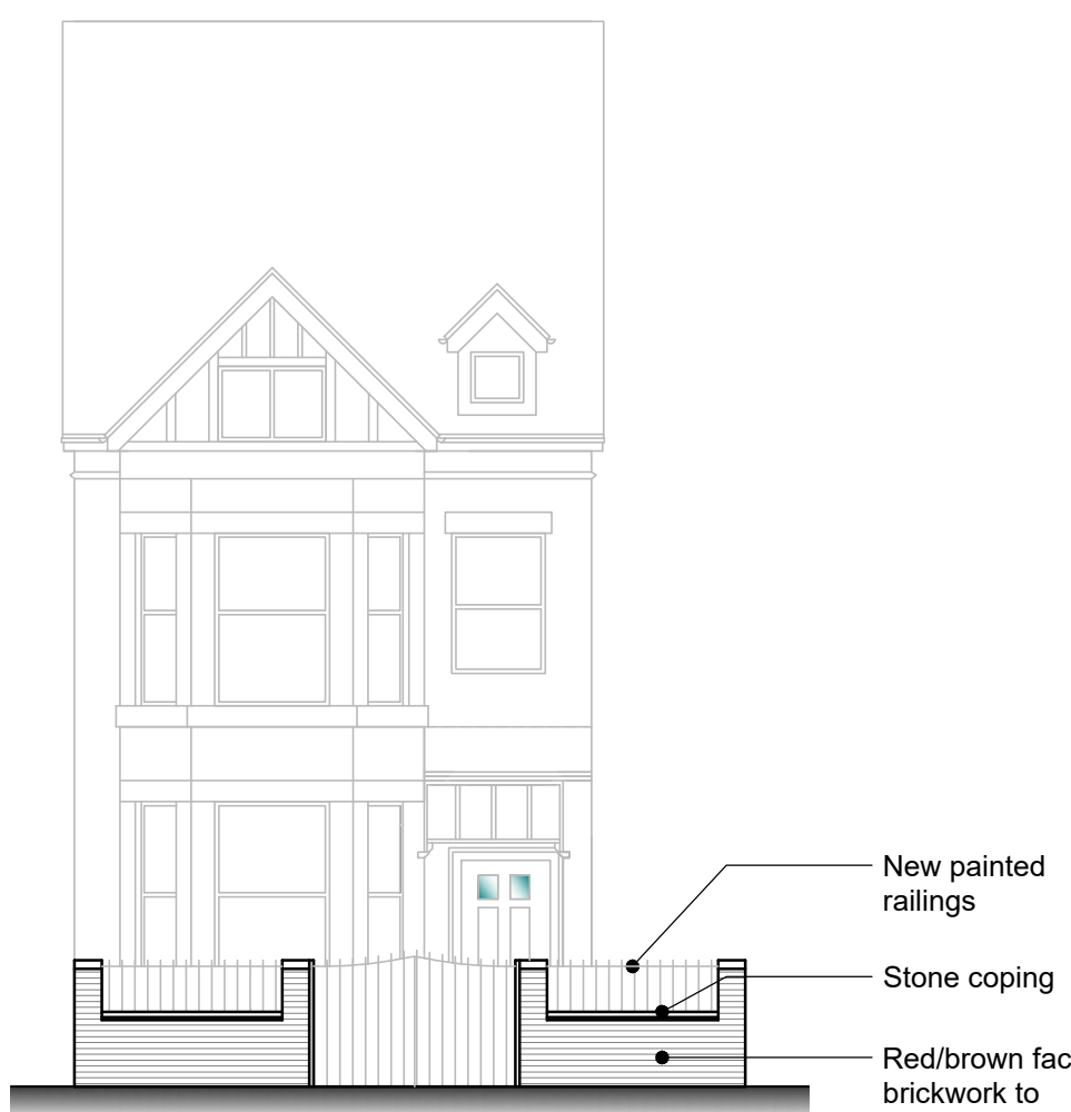
Proposed boundary wall elevation Scale 1:100
