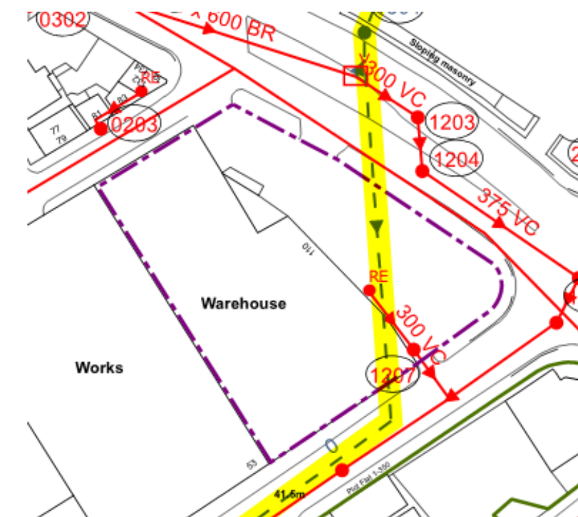
Figure 2.4 - United Utilities Sewer Records
