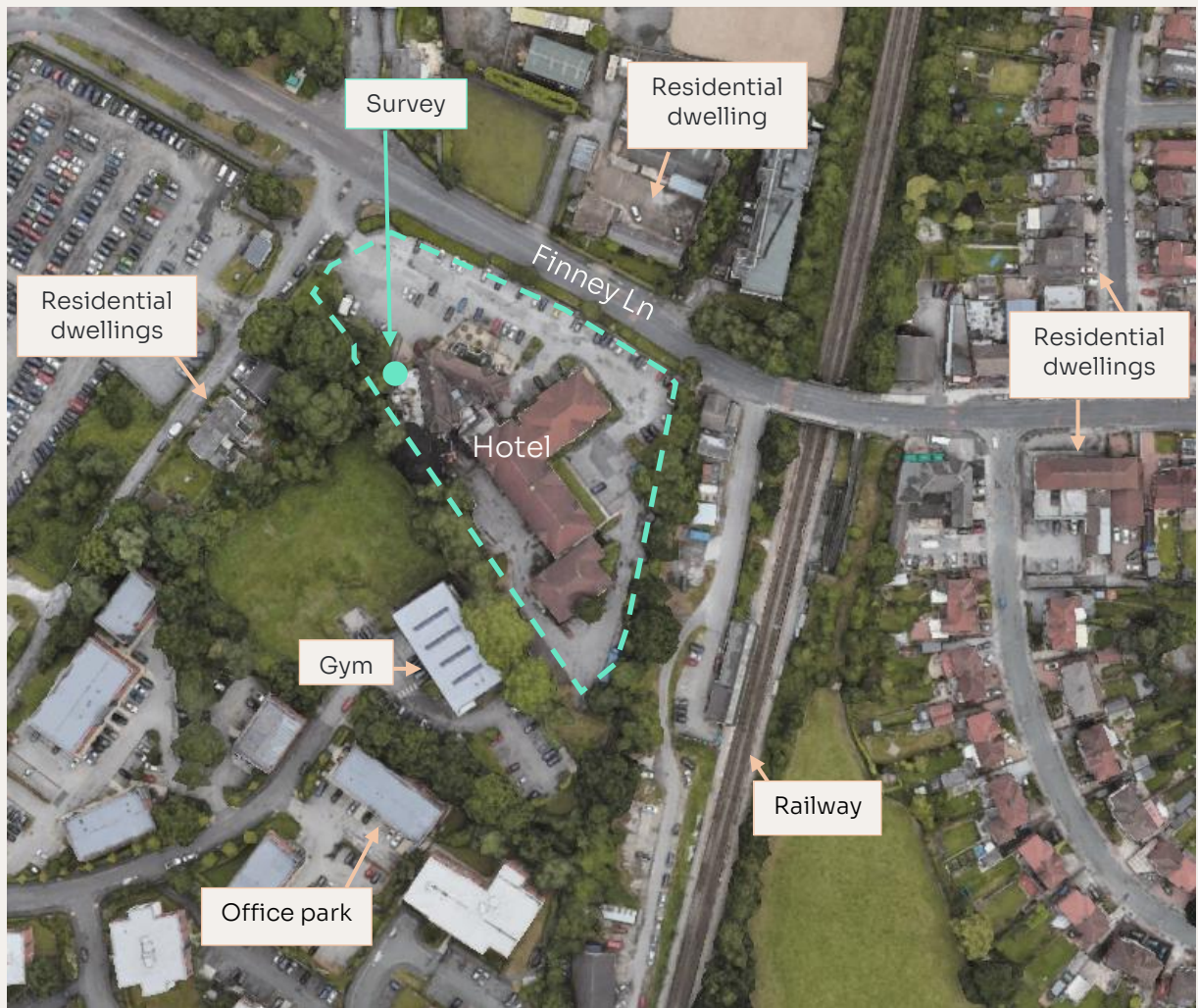
Figure 3-2 Aerial view of site, indicating local noise sources and properties which may be noise-sensitive. Satellite image courtesy of Google Earth.
