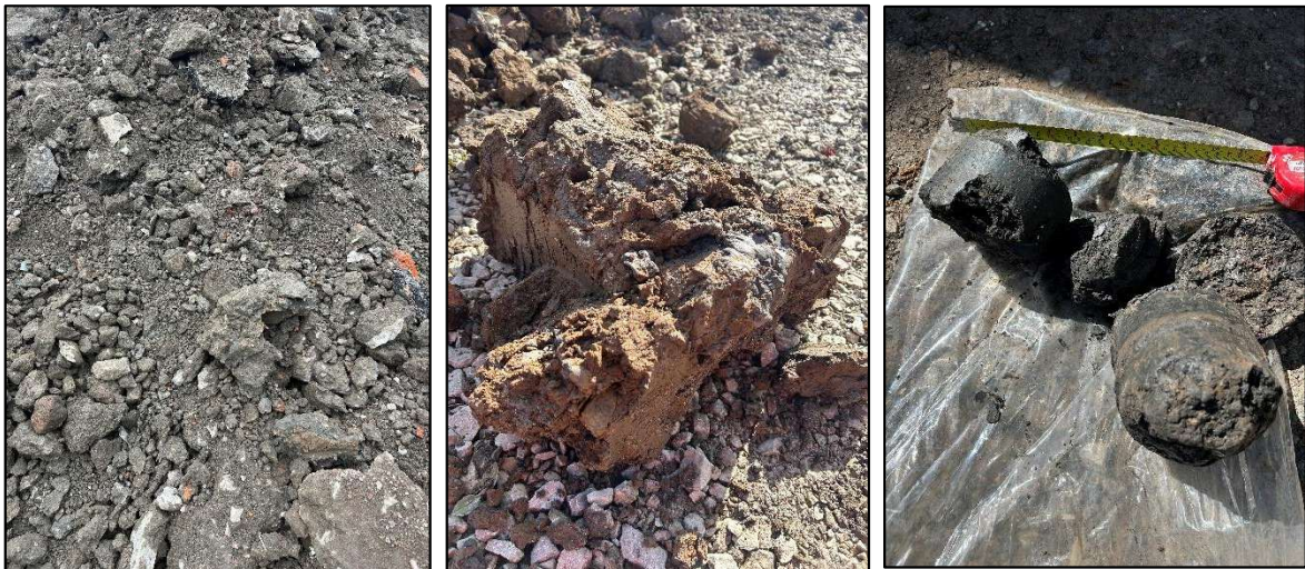
Figure 5: Typical Made Ground encountered in TP301 (left), typical Glacial Till encountered in TP305 (centre) and Pennine Upper Coal Measures in CP302 (right).
