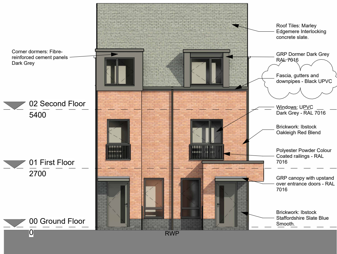
Front (North) Elevation 1 : 100
