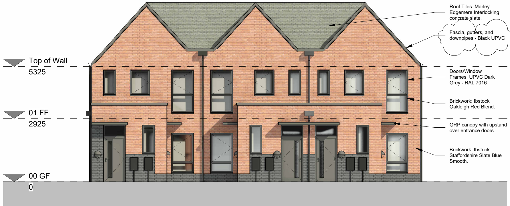
Front (North) Elevation 1 : 100
