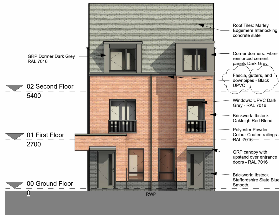
Front (North) Elevation
