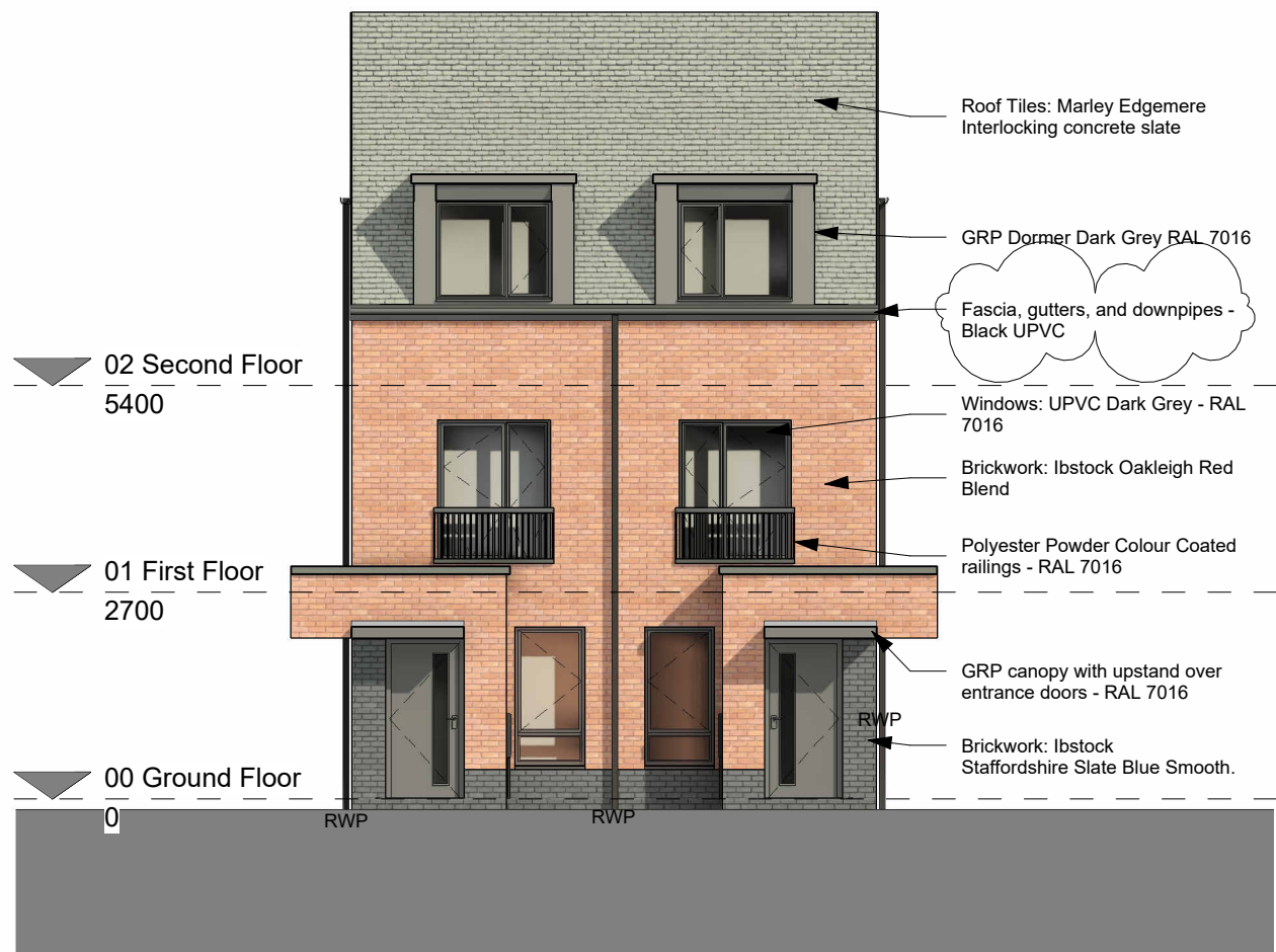
Front (North) Elevation 1 : 100
