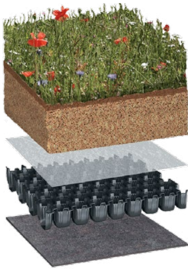
Typical extensive roof build up, 150-200mm deep
