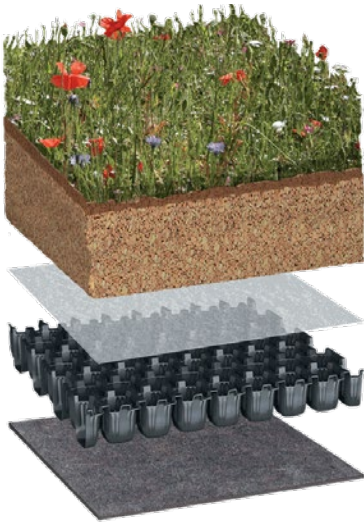
Typical extensive roof build up, 150-200mm deep
