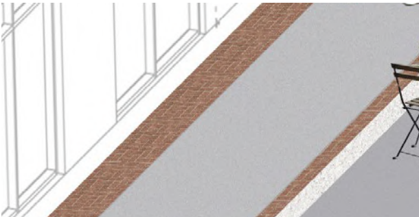
Paving bands to building edge and outer edge of the footpath with Tarmac surfacing infill
