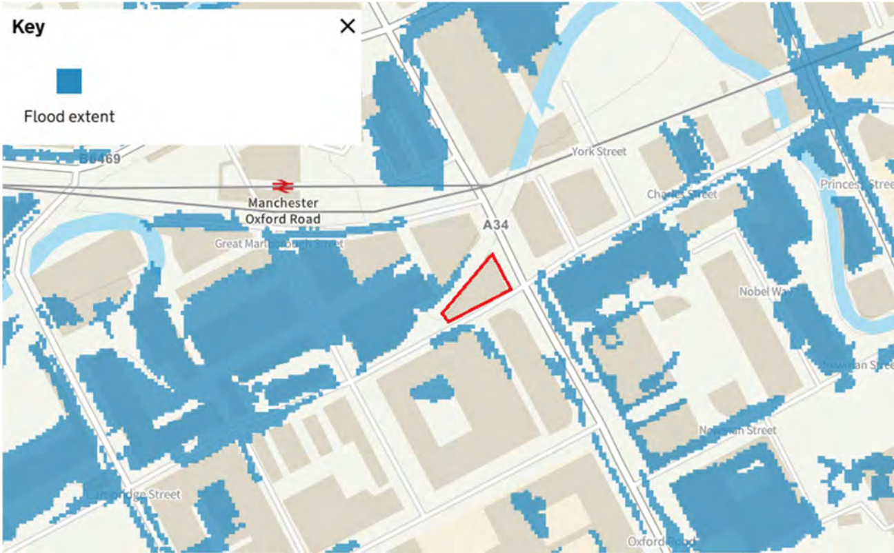
Figure 11. EA - Surface Water Flooding 1 in 100
