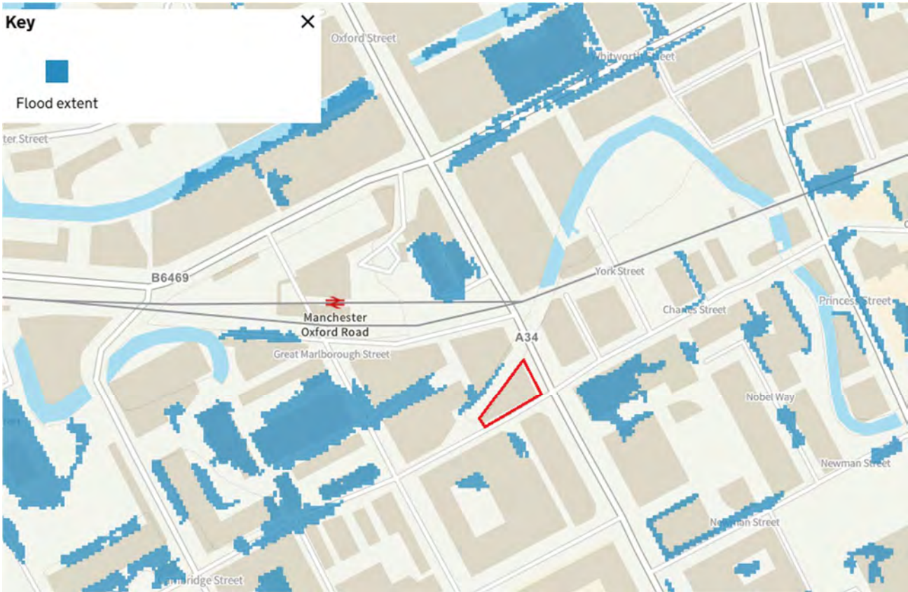
Figure 10. EA - Surface Water Flooding 1 in 100
