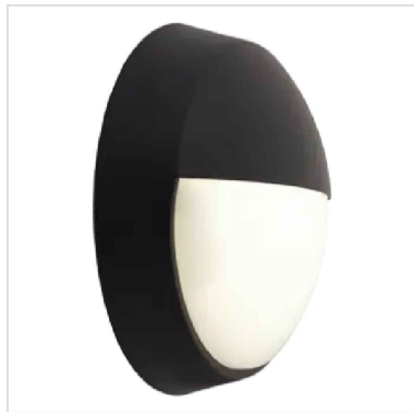
ABOVE: F1E - EXTERNAL SURFACE EYELID LED BULKHEAD WITH 3 HOUR EMERGENCY BATTERY BACK UP PACK - SIZE: 215MM DIAMETER X 80MM DEPTH - POSITIONED APPROX 2.5M ABOVE EXTERNAL GROUND LEVEL
