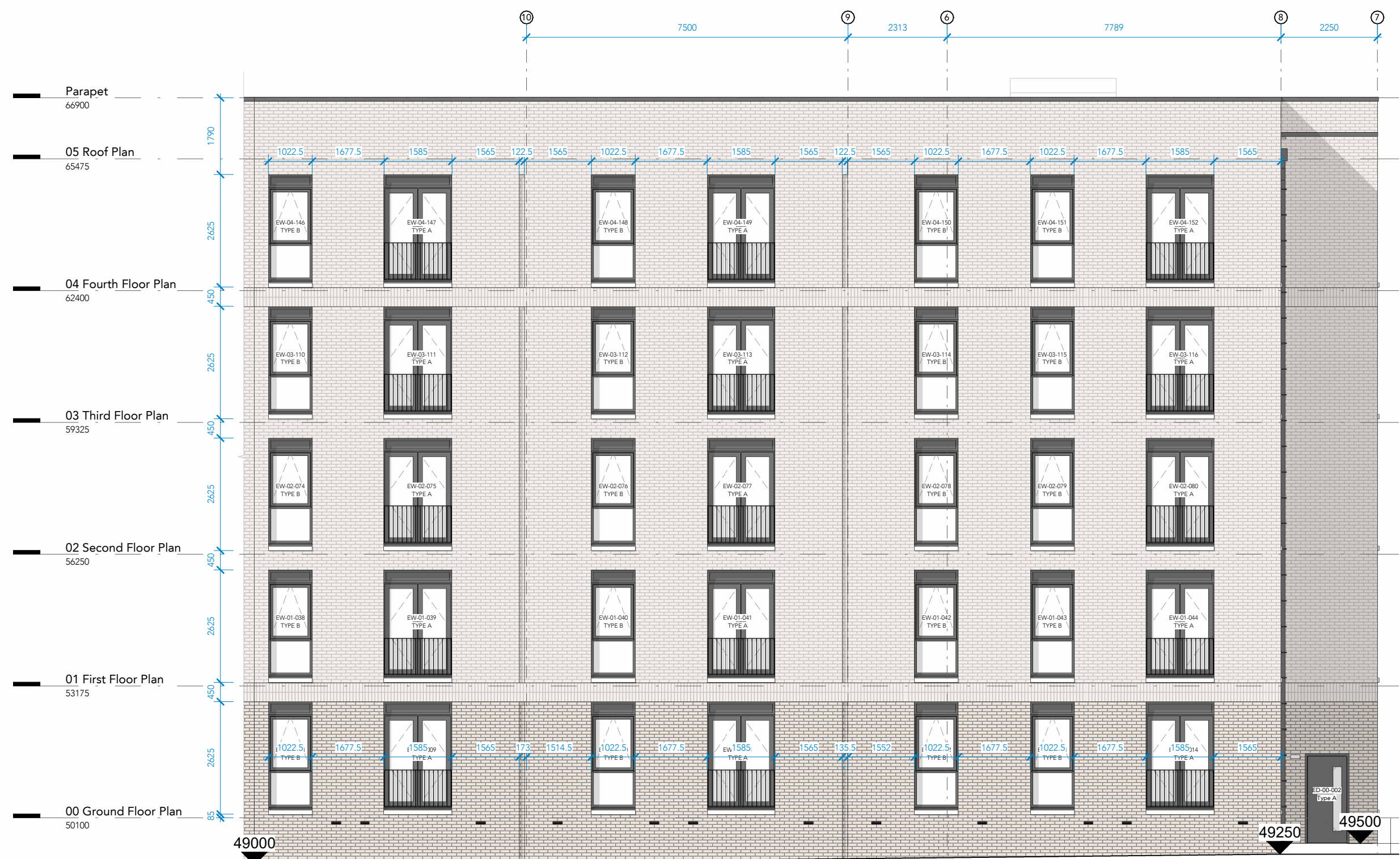
East Elevation 2 - General Arrangement 1 : 100
