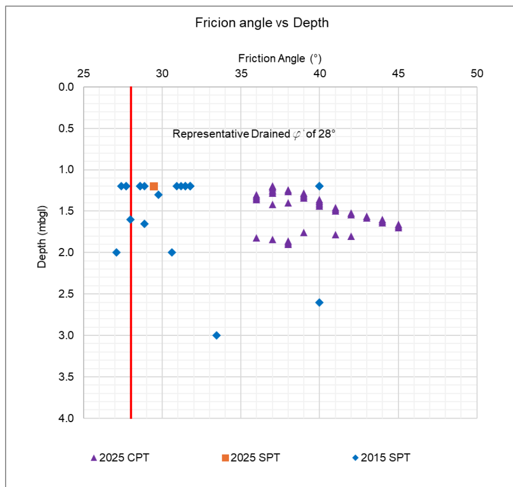
Figure 4-2: Friction angles derived for the Made Ground based on SPT and CPT
