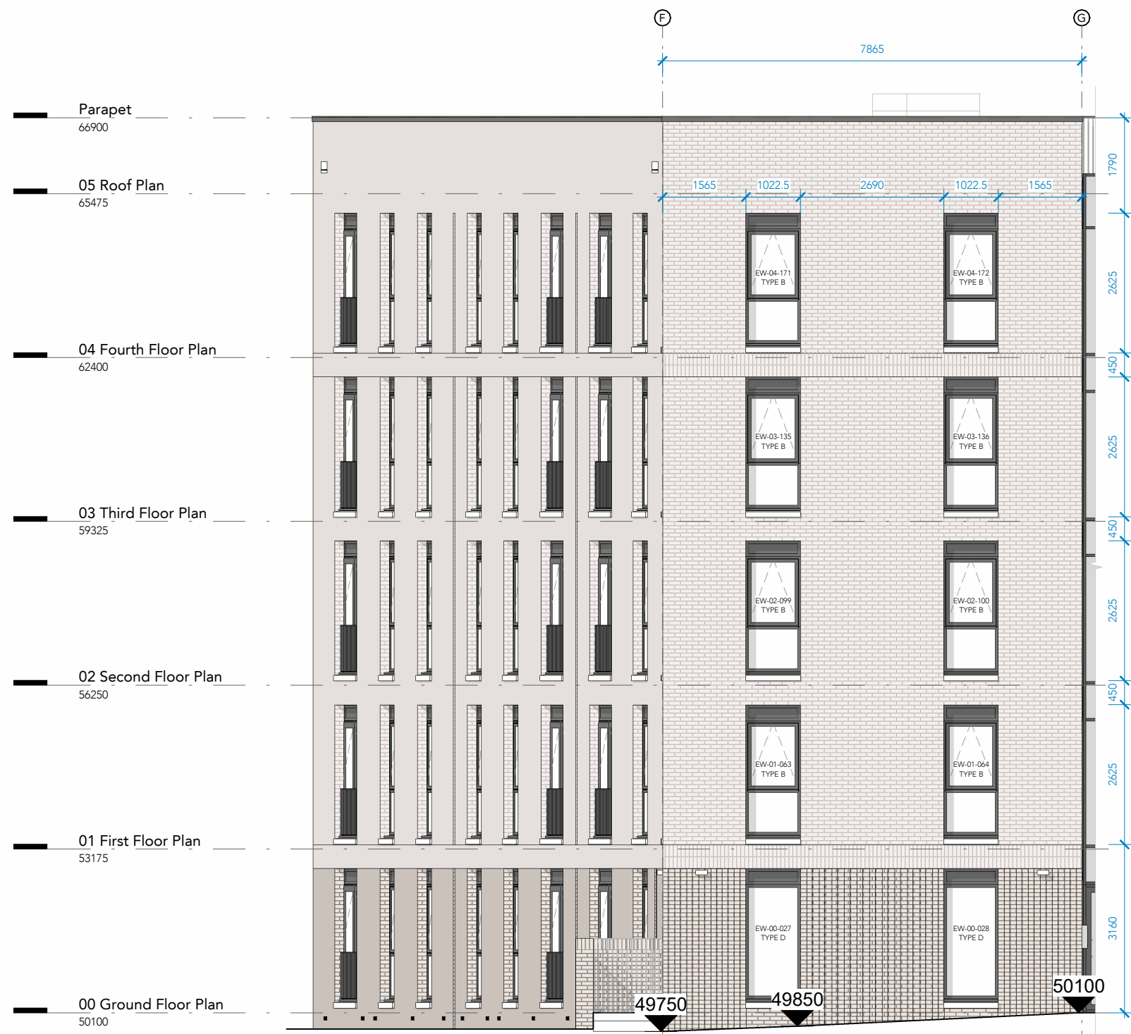
South Elevation 1 - General Arrangement
