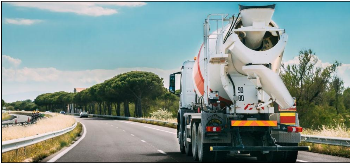
Figure 3. Transport of concrete from manufacturing plant to construction site. Transport of materials to site typically accounts for around a tenth of the total upfront carbon impact (A1-A5).
