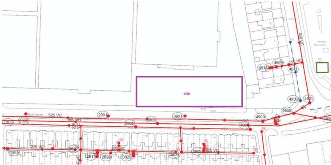
Figure 3 – United Utilities Sewer Records
