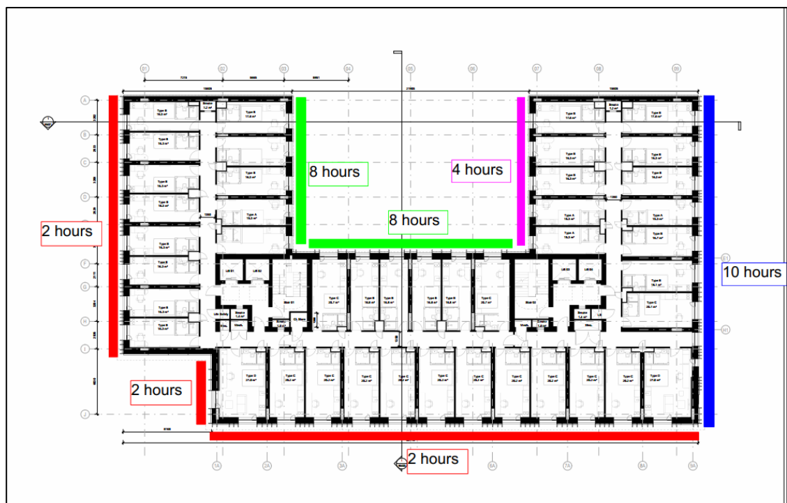
Figure 3: Maximum allowable daytime opening duration of windows and purge vents, Levels 1 to 12
