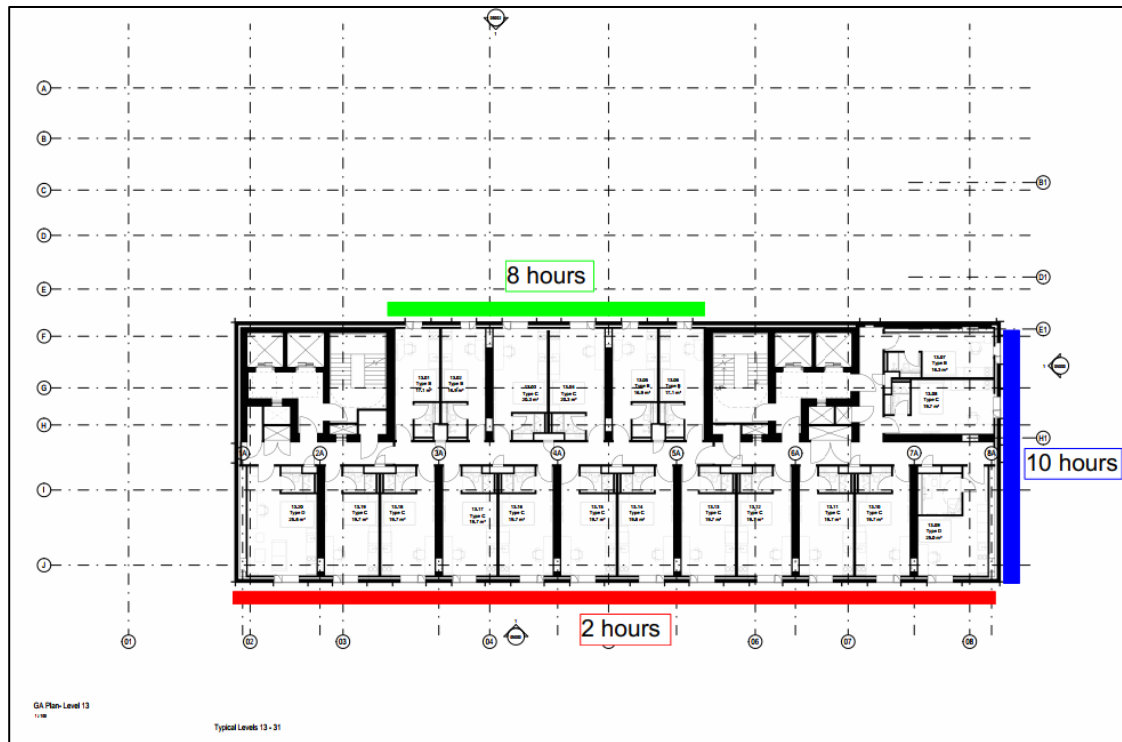
Figure 4: Maximum allowable daytime opening duration of windows and purge vents, Levels 13 to 31
