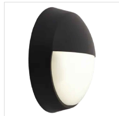
ABOVE: F1E - EXTERNAL SURFACE EYELID LED BULKHEAD WITH 3 HOUR EMERGENCY BATTERY BACK UP PACK - SIZE: 215MM DIAMETER X 60MM DEPTH - POSITIONED APPROX 2.5M ABOVE EXTERNAL GROUND LEVEL
