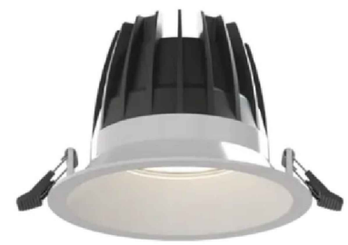
ABOVE: V - IP65 RATED EXTERNAL LED CANOPY WARM WHITE LIGHT - SIZE: 140MM DIAMETER X 95MM HIGH - POSITIONED WITHIN GROUND FLOOR SOFFIT
