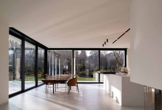
13.1.01 Reynears SL38 Fixed aluminium framed glazed window Standard RAL 9005 black frame finish
