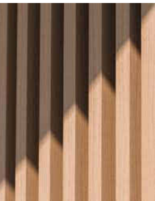
7.1.01 Knotwood Cladding Privacy Panel 25mm x 25mm Knotwood vertical aluminium cladding with a maximum spacing of 7mm fixed to Knotwood horizontal mounting track. Natural Oak finish.
