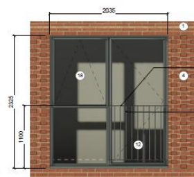
Top Storey Window Bay Detail
