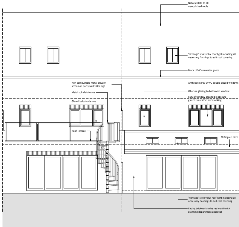
Rear Elevation - Plot 3 (Roof Terrace)
