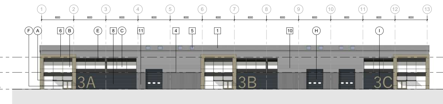
3 Proposed South Elevation Scale @ 1 : 200
