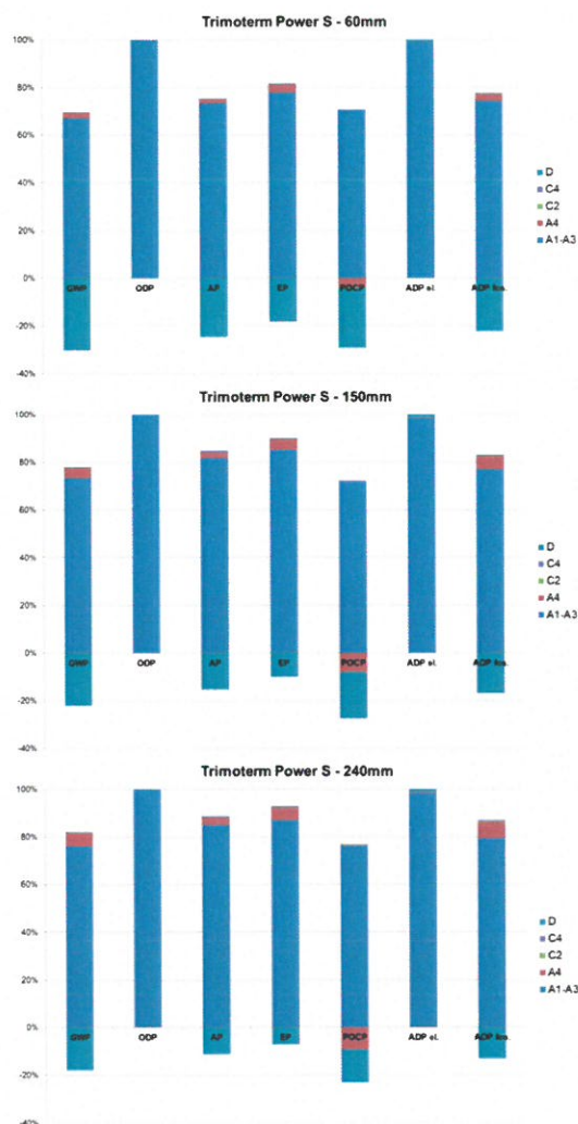
Figure 3: The relative contributions of different life cycle stages (i.e. modules A1-A3, A4, C2, C4 and D) to the environmental impact of Trimoterm Power S façade panels
