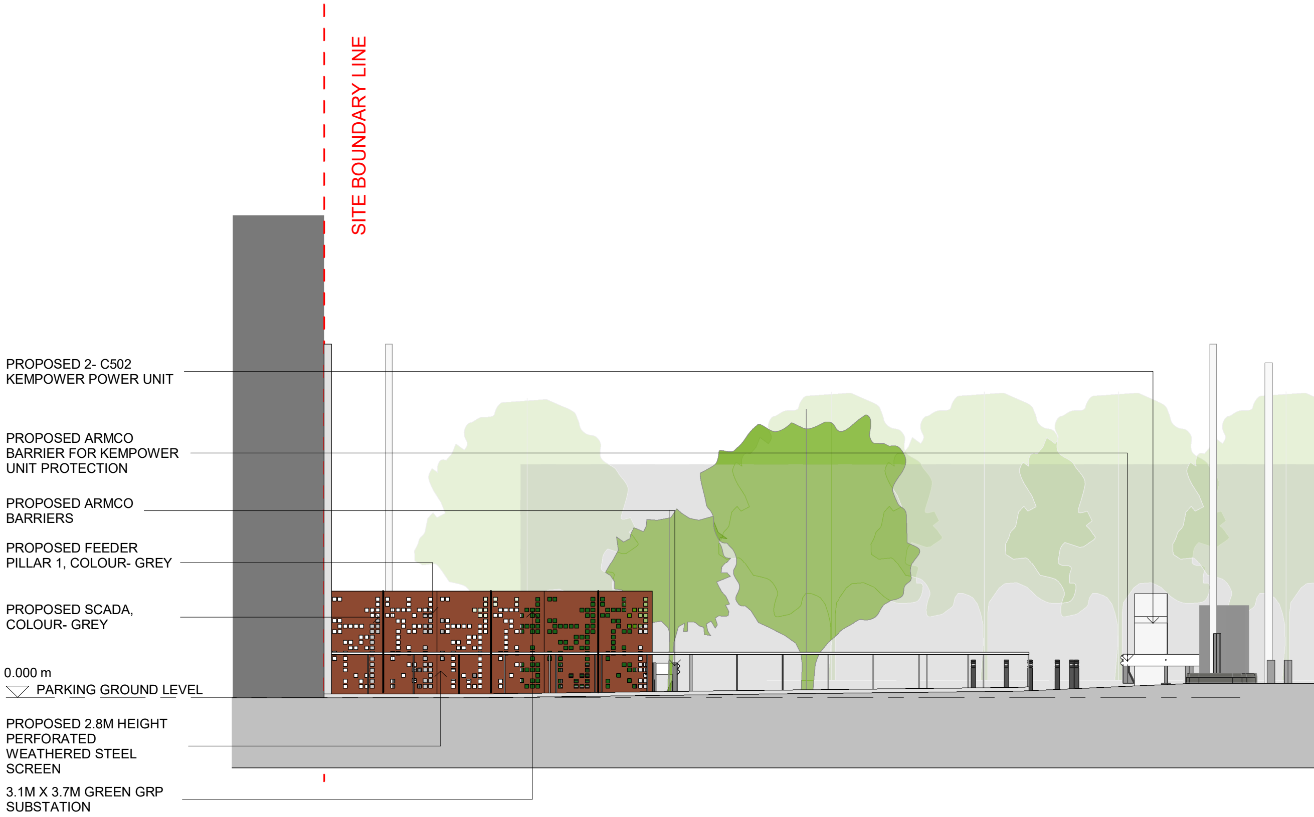
PROPOSED SITE ELEVATION C-C FROM BLOOM STREET 1 : 100
