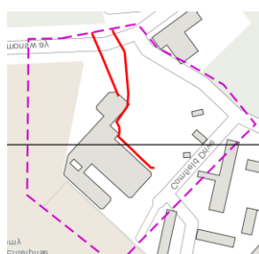
EXA fibre optic isolated and removed.
