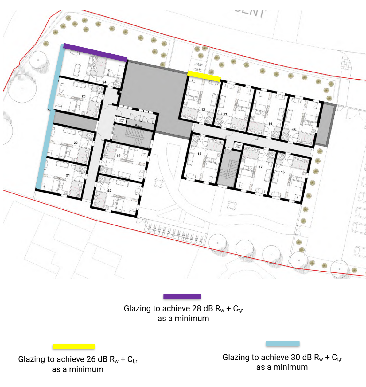
FIGURE 5.2 LOCATION OF HIGHER SPECIFICATION GLAZING (FIRST FLOOR)
