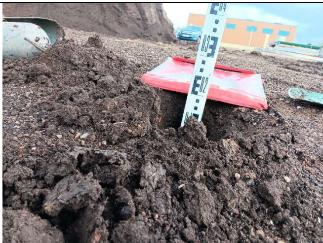
Depth measurement HD117 ( circa 200mm soil cover over membrane).
