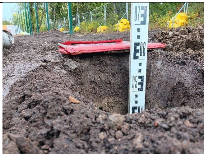
Depth measurement HD106 ( circa 630mm soil cover over membrane).
