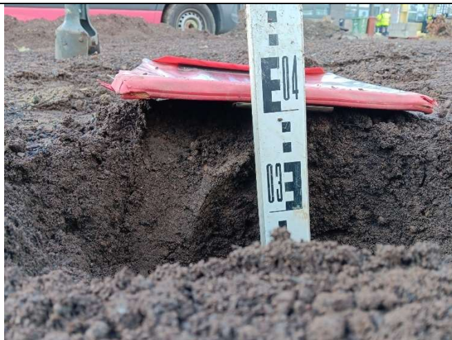
Depth measurement HD105 ( circa 400mm soil cover over membrane).
