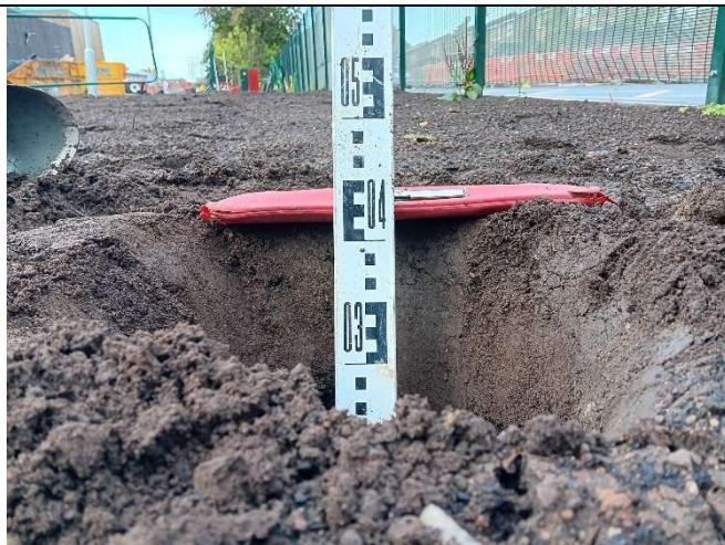
Depth measurement HD104 ( circa 420mm soil cover over membrane).
