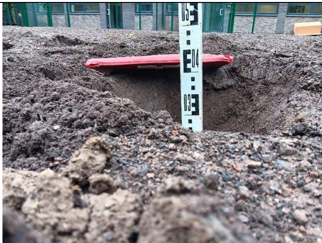
Depth measurement HD107 ( circa 420mm soil cover over membrane).
