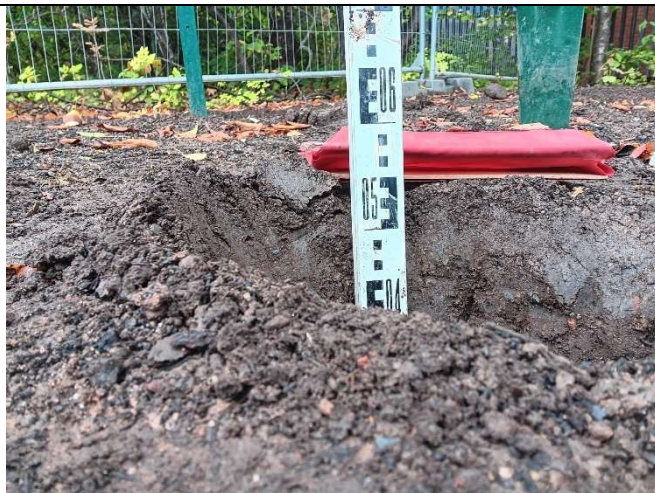
Depth measurement HD108 ( circa 550mm soil cover over membrane).
