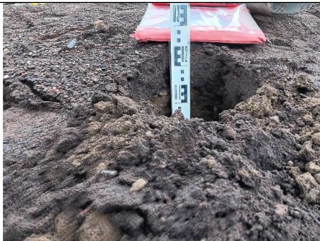
Depth measurement HD116 (circa 250mm soil cover over membrane).
