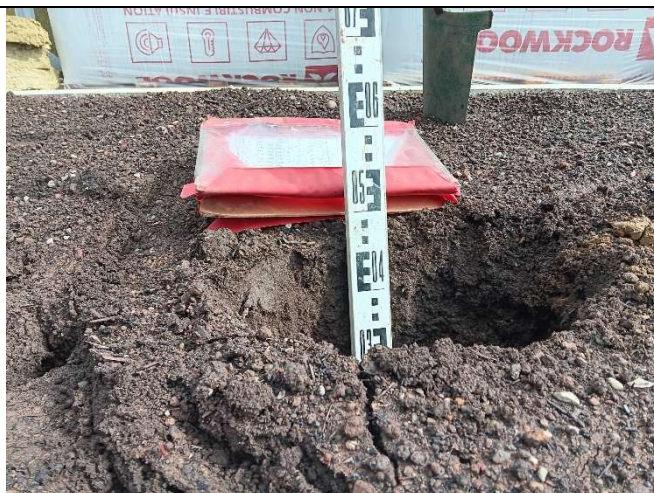
Depth measurement HD118 (circa 500mm soil cover over membrane).
