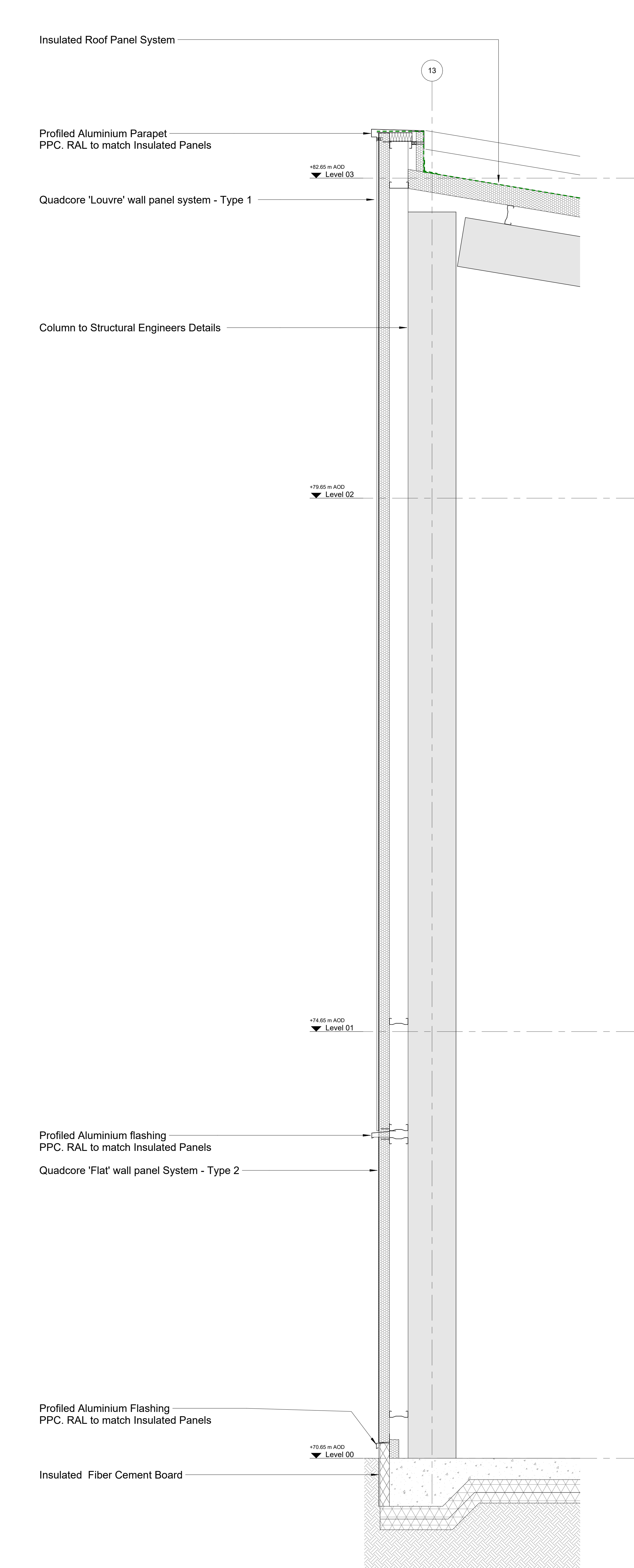
1 Typical Strip Section - Gable End 1 : 20
