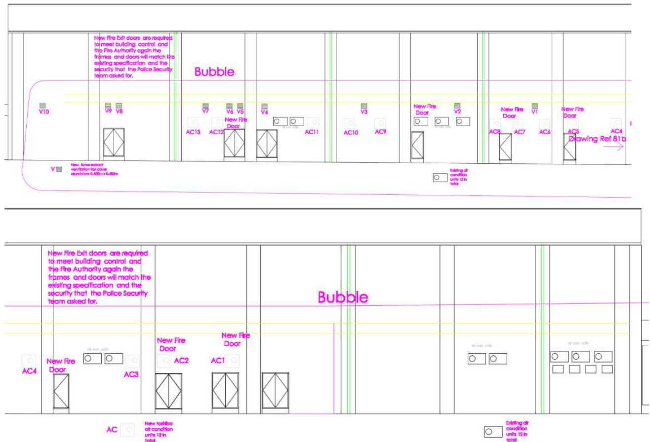
Figure 1.2 Locations of Installation on Northern Façade
