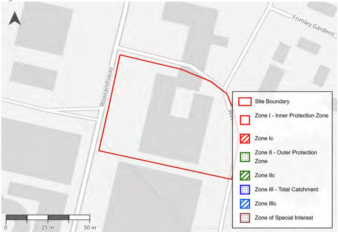
Figure 2.5: Groundwater Source Protection Zones
