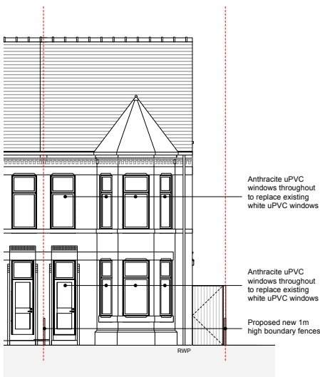
Proposed Front Elevation 1:200 Scale
