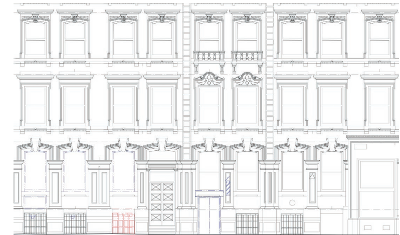
Image: Showing proposed areas of removal of historic fabric (in red) and proposed areas of removal of non-historic fabric (in blue).
