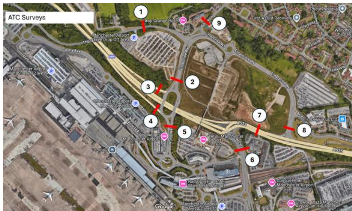
Plate 11.3: Automatic Traffic Count (ATC) Locations
