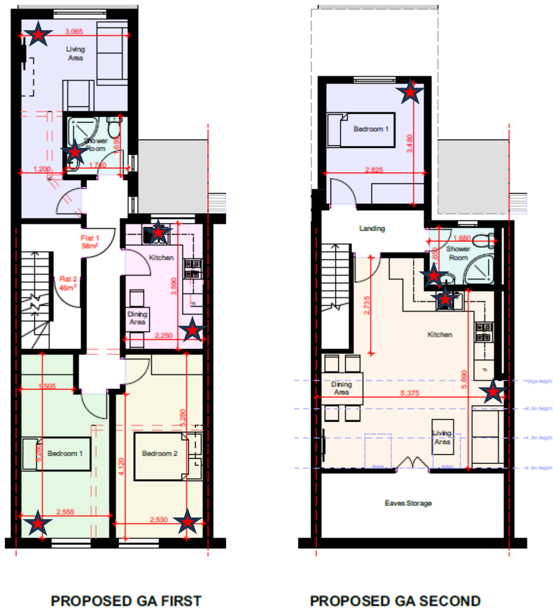
Plate 1: Internal bin potential storage locations
