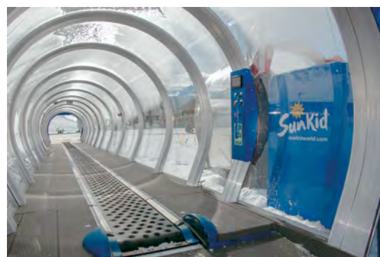
Operation terminal inside the gallery
