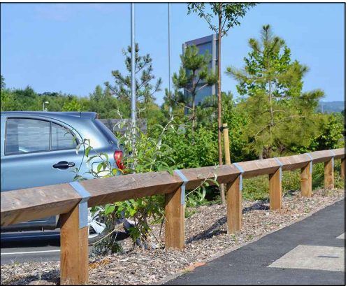
BARRIER Type 2 - Knee rail Timber knee rail
