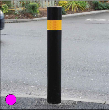
BOLLARD Type 3 - Impact Protection Heavy duty steel posts, 950mm high, 114mm dia Root fixed
