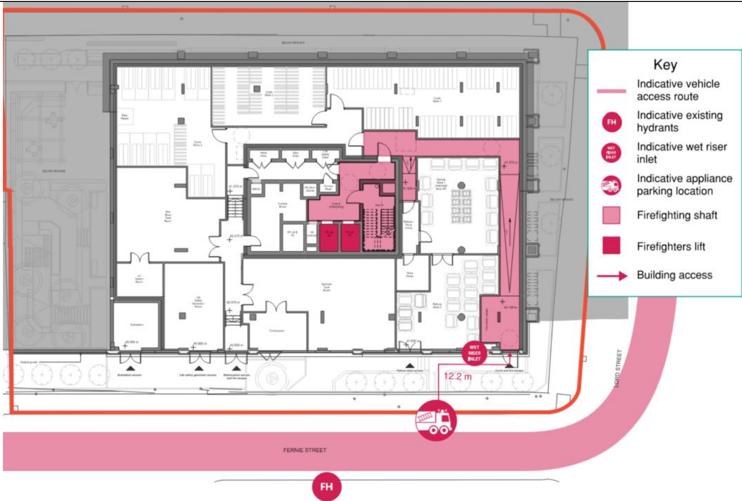
Figure 3: FRS site access and hydrant provisions (basement)
