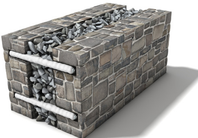
Stabilising a cracked rubble-filled wall.
