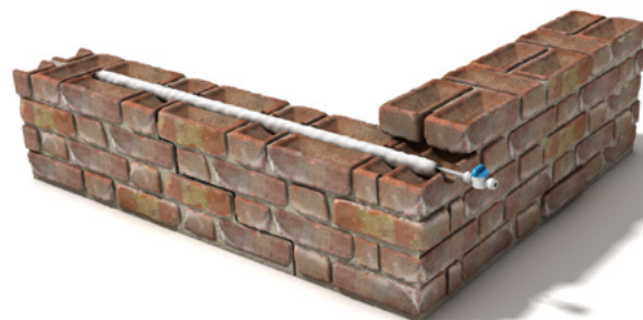
Stitching a cracked solid wall.
