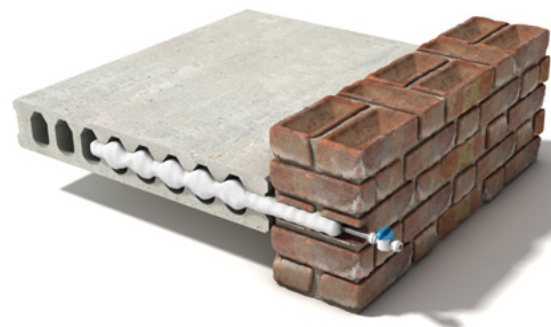
Securing an external wall to a hollow concrete floor slab.
