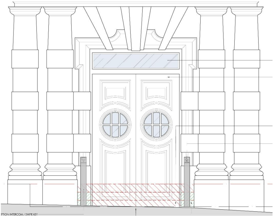
Fig 10: External elevations, showing existing doors relocated with fanlight above, and door controls/voice communication points provided on freestanding external stainless steel posts
