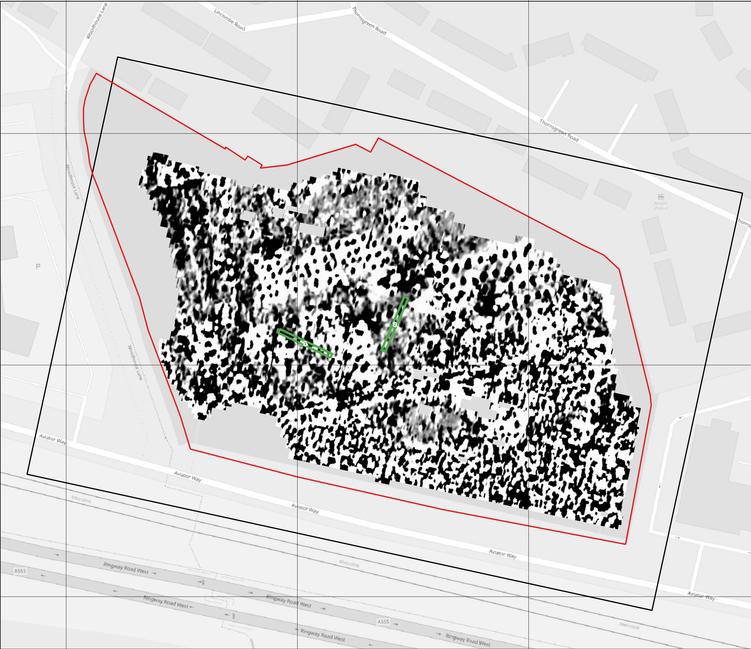
Figure 3. The proposed trench locations overlain on the preliminary geophysical greyscale
