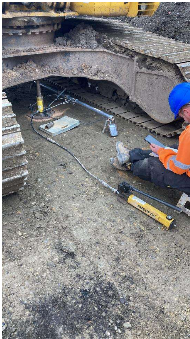
NT03 pile mat: final deformation plate tests
