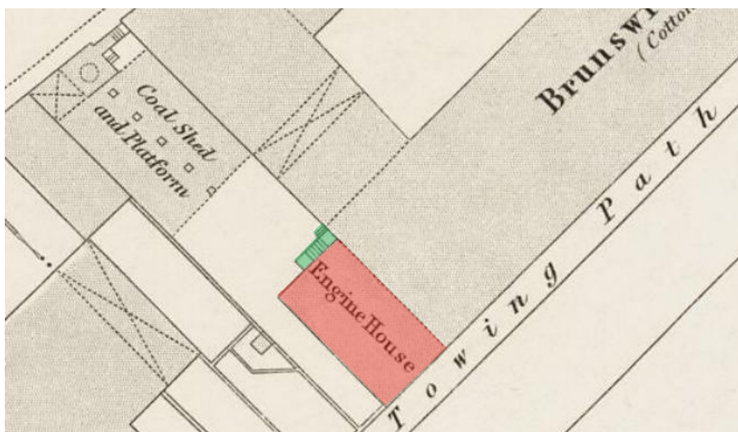
Figure 3 - The 1851 OS map shows the “Engine House” located within a yard area containing the mill chimney, a coal shed and a platform parallel with Bradford Road next to the original location of the mill’s boilers which were housed within the ground floor of the mill.
