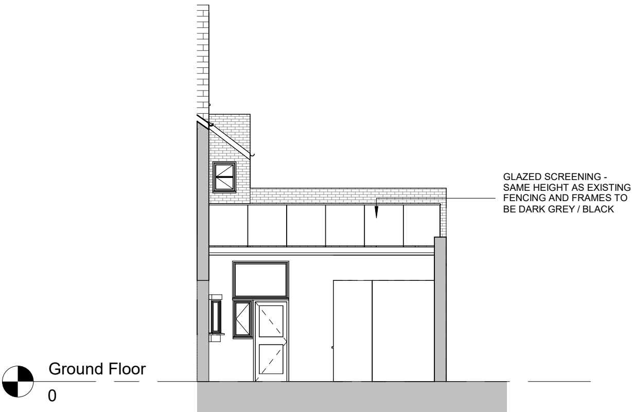
5 ELEVATION - FRONT ENTRANCE BELOW ROOF TERRACE 1 : 100
