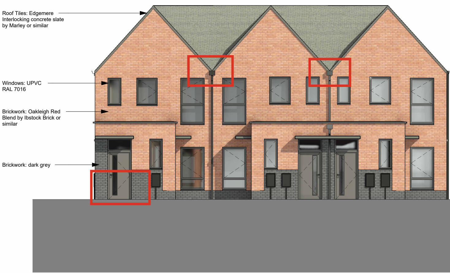
Front (North) Elevation 1 : 100
