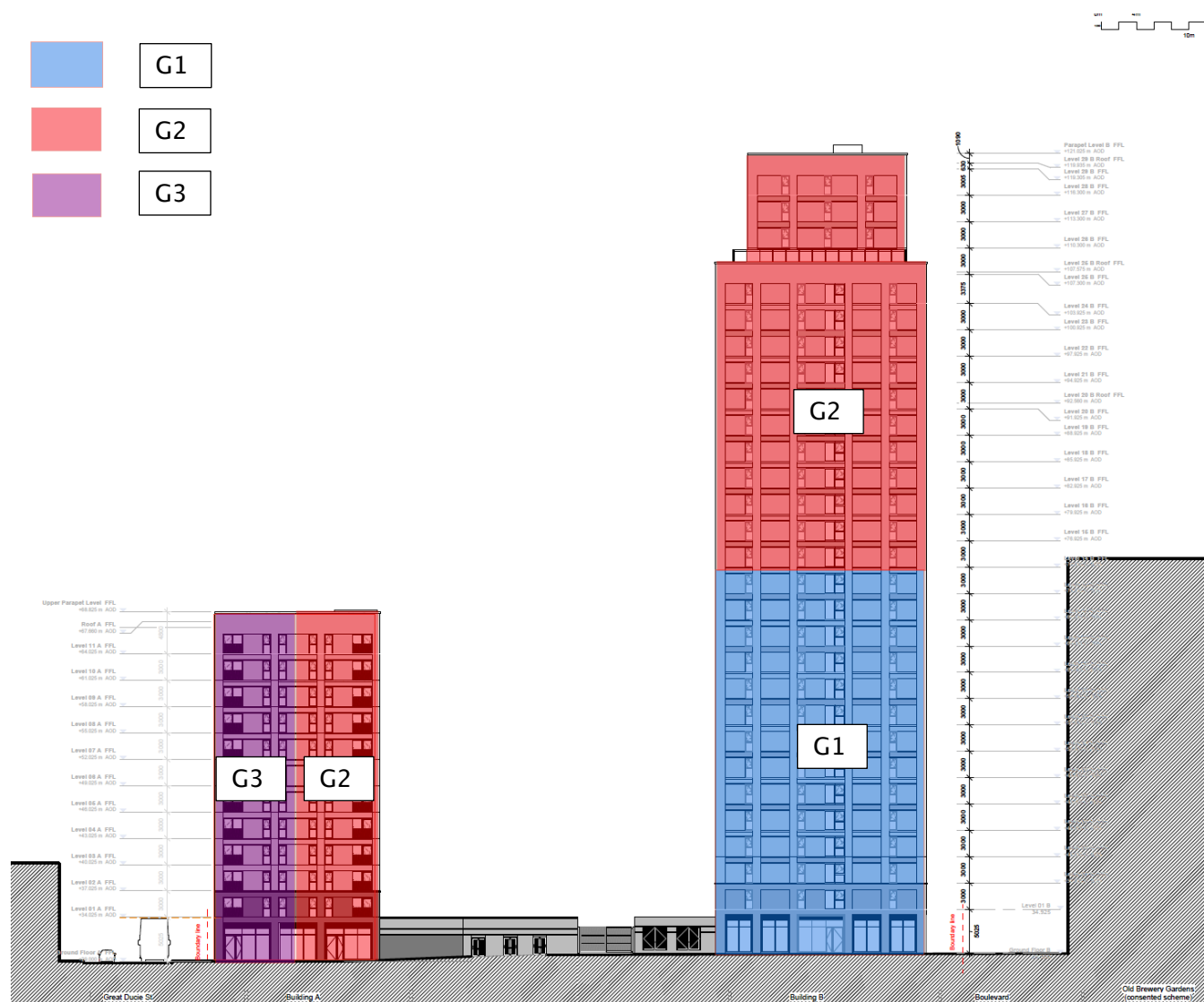
Figure 3.4: Glazing Requirements – South Facing (towards AO Arena)
