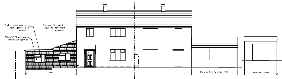
04 PROPOSED FRONT ELEVATION Scale 1:100 @ A1
