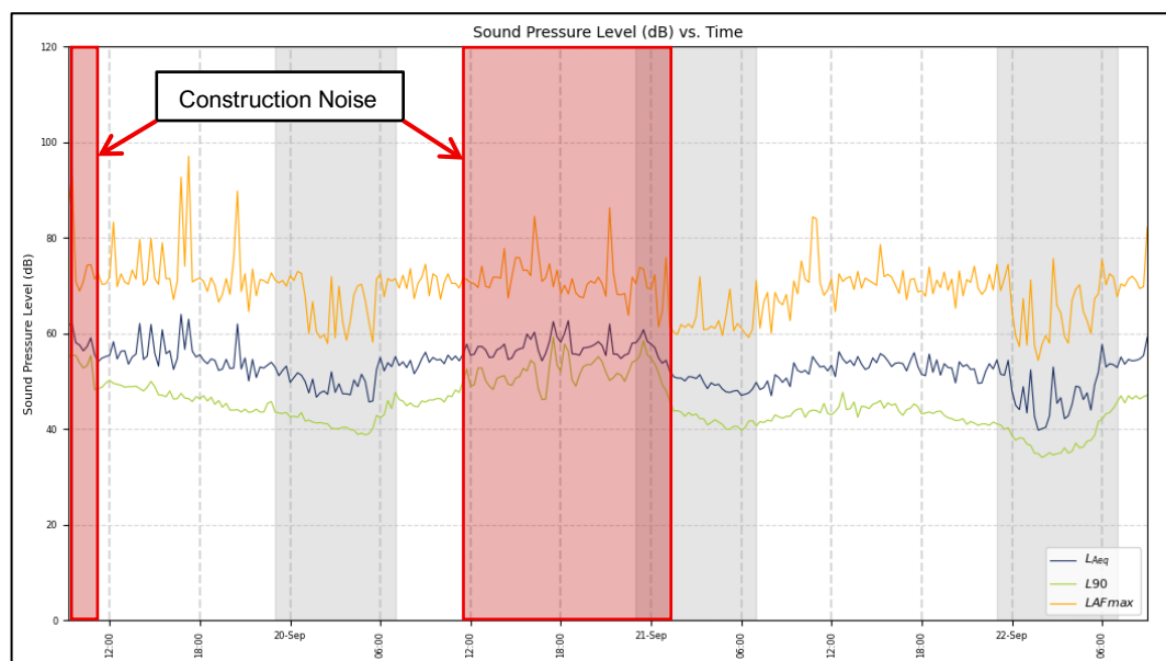
Figure 5: Level vs. time graph showing L_{Amax} , L_{Aeq} and L_{A90} sound levels – ML1
