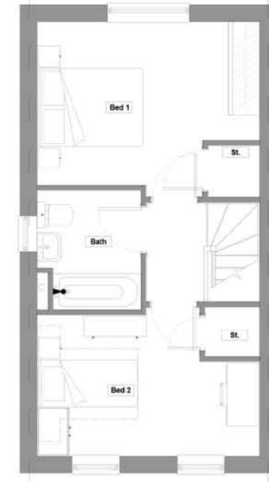
First Floor Scale - 1:100
