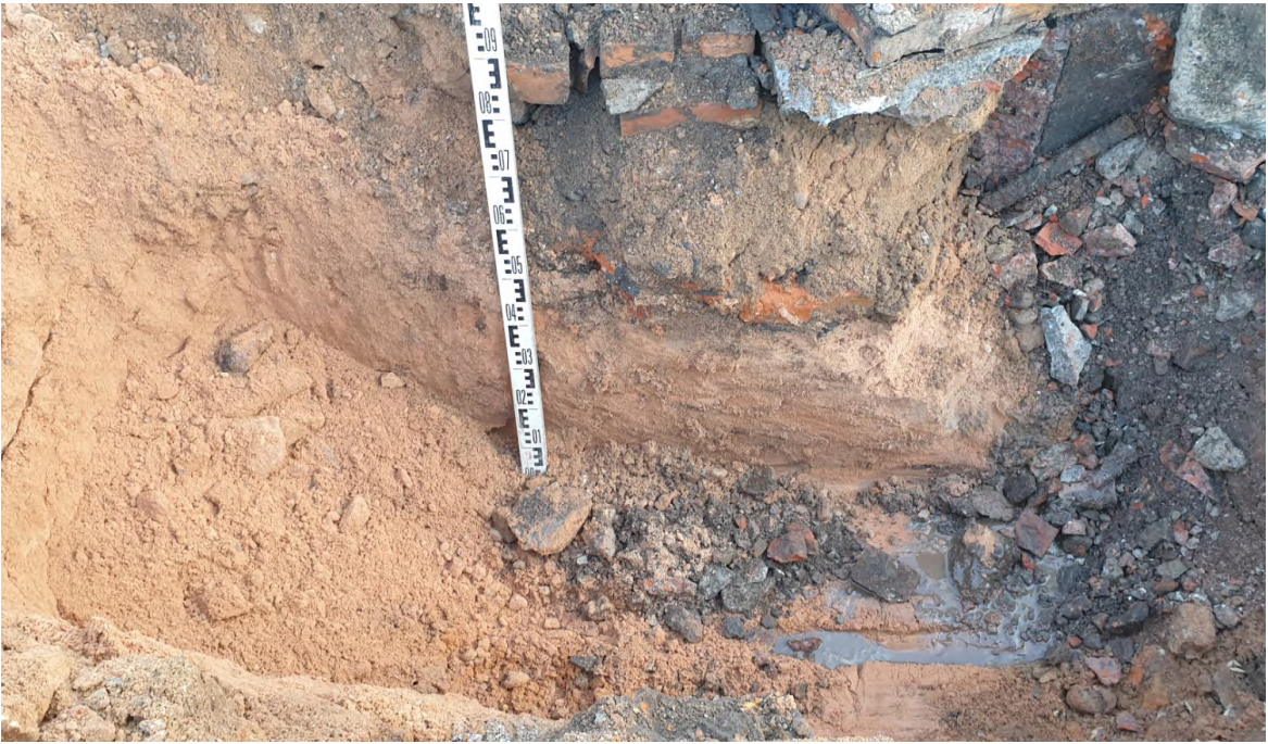
Soil sample obtained for leachate analysis in pit at depth of 1.00m
